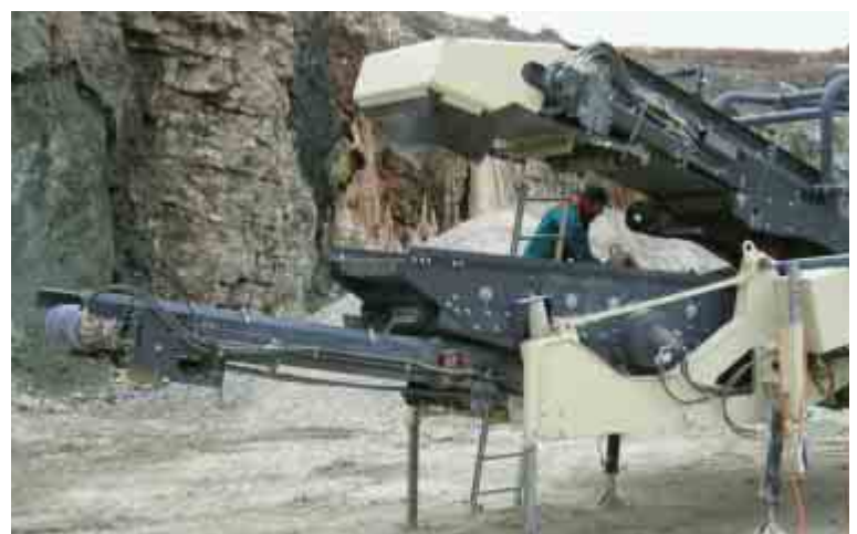
The screen of Lokotrack LT1213S can be opened easily for servicing and screen mesh change using the hydraulic system.
