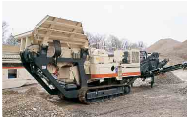
Sturdy, 4m 3 or 6m 3 Hardox steel feed hoppers can be chosen for the Lokotrack LT96S.
