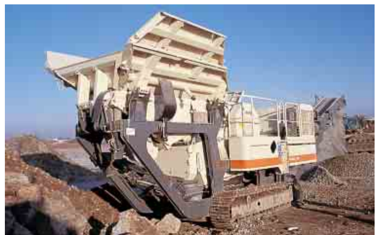
Another unique Lokotrack LT96 feature is the automatic locking mechanism for the feeder, cutting the time needed to prepare for transportation.
