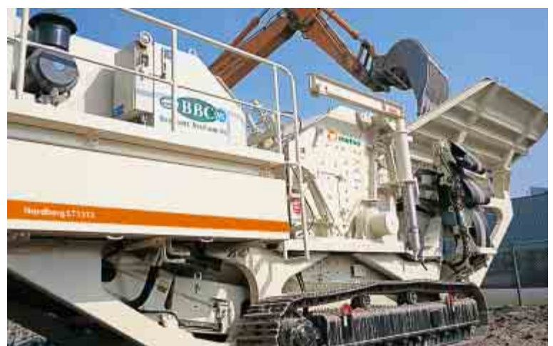
The new, Nordberg NP1213M impact crusher has been developed for the Lokotrack LT1213 mobile crushing plant.
