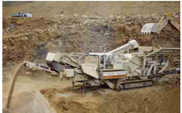
Lokotrack LT1213S crushing and screening limestone in France.
