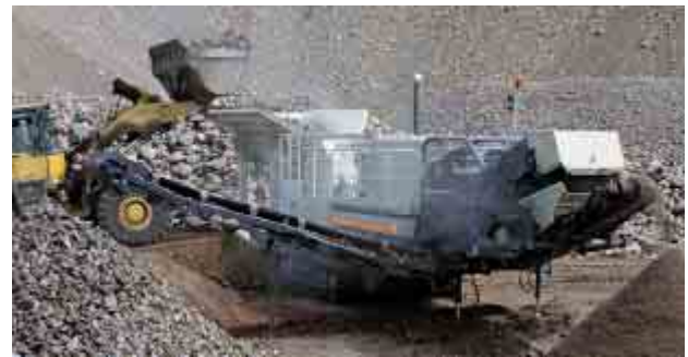
Lokotrack LT105S jaw plant with a detachable screen.
