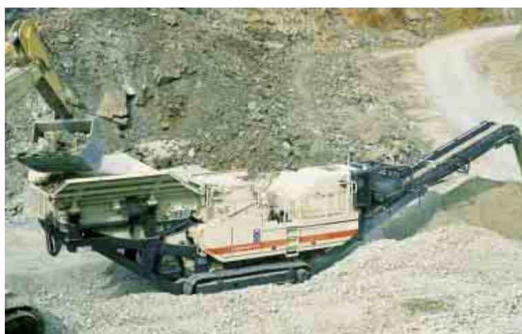
New design using separate elements result in lower operating noise levels.
