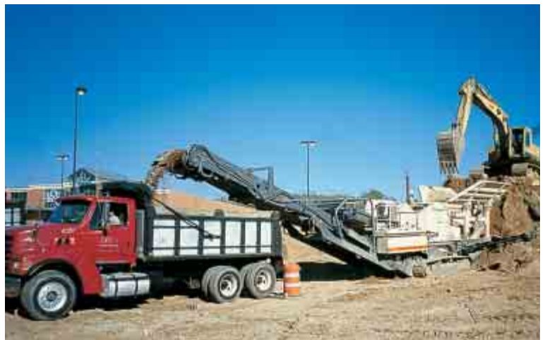
Lokotrack LT105 equipped with an extra long 12 metre conveyor crushing in the USA.
