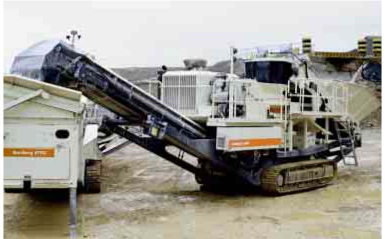
Lokotrack LT200HP can be easily operated with a primary impactor or jaw plant and with a mobile screen.
