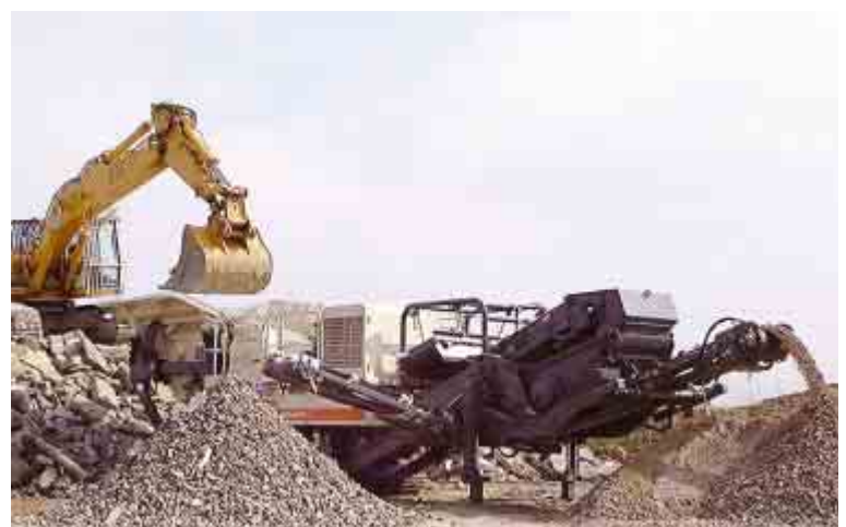
The Lokotrack crushing recycled concrete in Germany.
