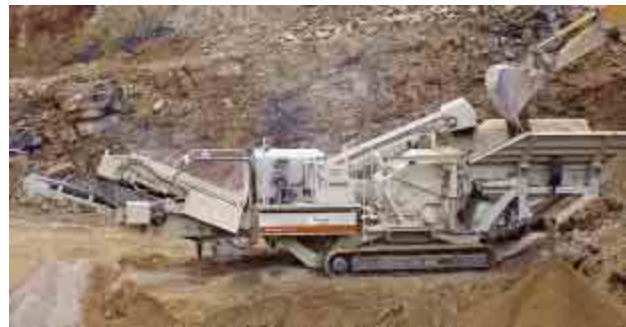
Lokotrack LT1213S impactor plant with a detachable screen.
