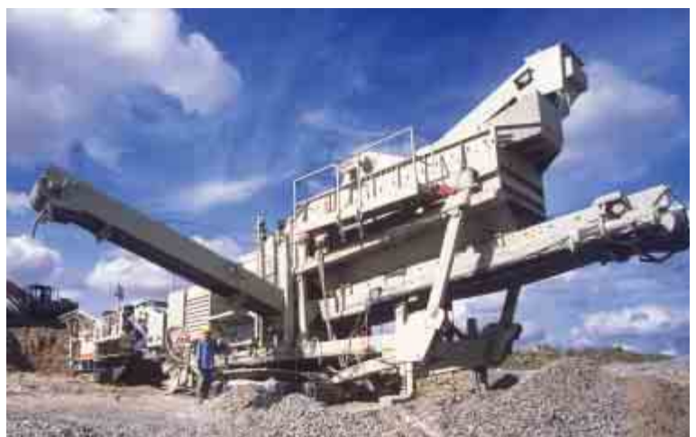
Nordberg GP11M or GP11F cone crushers can be selected to LT1100.
