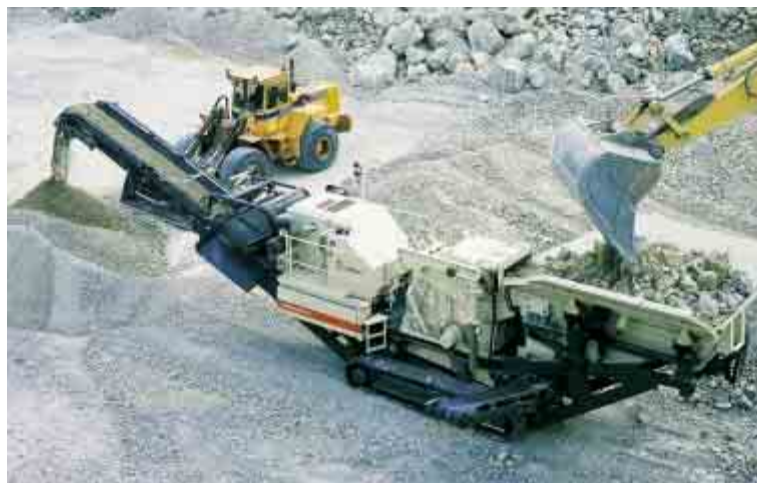
According to the application, Lokotrack LT1110 can be equipped with 5m 3 or 8m 3 sized feed hopper.
