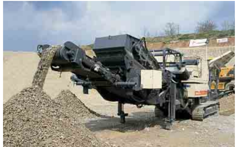
The detachable screen of the Lokotrack LT96S guarantees efficient classifying of the crushed materials into clean end products.
