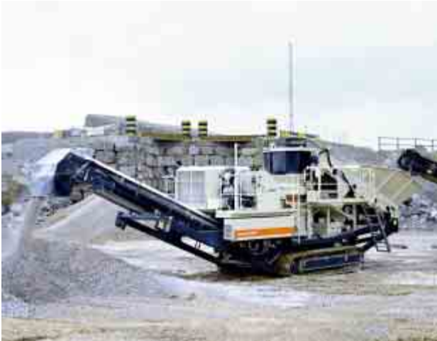
Lokotrack LT200HP cone plant.
