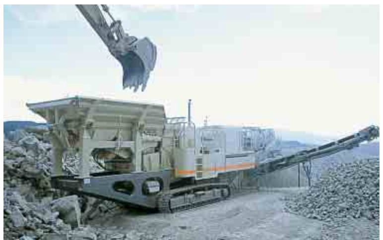
The Lokotrack LT105S side conveyor is easily tilted for transport.
