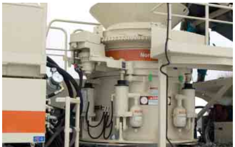
LT200HP is built around the proven and popular HP200 cone crusher.
